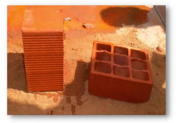
Porotherm Smart Bricks can be cut into desired sizes using wet cutting machine used commonly for granite/ marble cutting
